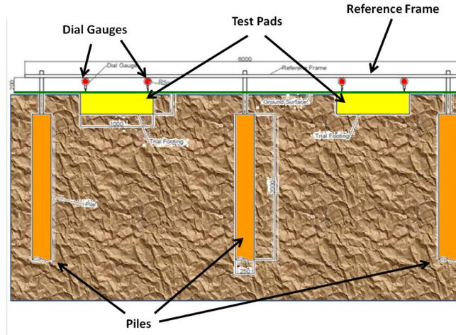
Above, a section through the test site showing the location of the concrete pads (shaded yellow) and the reference frame supported on piles. Below, a plan of the installation showing the arrangement of the electrodes at each of the test pads. One set of electrodes were installed vertically and another at an angle. A third used intermittent current and the fourth was a control with no treatment applied.
