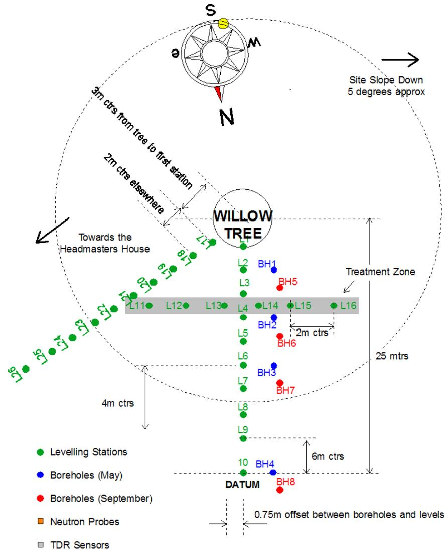
*The existing level stations may be a target for further EKO treatment to understand the response both in the area of treatment and beyond. In theory EKO treatment will stabilise the soil at (possibly isolated) treated stations and shrinkage/swelling should be minimal. How will the level stations distant to the treatment zone respond? The benefit here is the ability to compare the effect with historic readings.*
